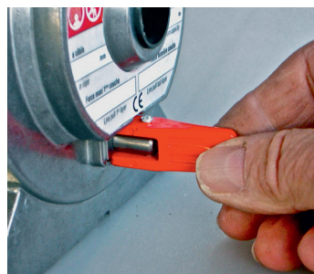
➤ Disengageable drum, no load only.
